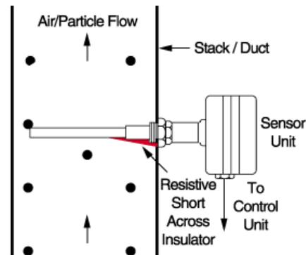
In Electrodynamic systems this problem can be minimised by using a completely insulated probe (sensor rod is insulated over full length) which has no resistive path to ground. The insulated probe continues to measure in spite of its insulated coating since the induction phenomena does not require direct contact between particles and sensor rod. The insulated probe is covered by separate PCME patents.
