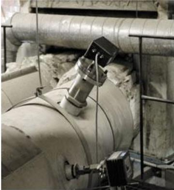
Figure 6 Electrodynamic sensor fitted in incineration process after ceramic filter
