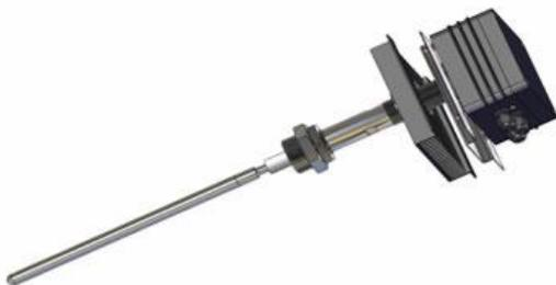
Figure 4 High temperature Electrodynamic particulate sensor capable of monitoring in stack temperatures to 1200°C
