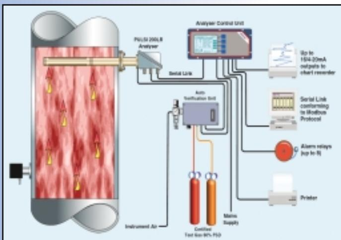
The calculated concentrations can be displayed on a PC or weatherproof industrial PC. Up to four analysers can be connected to the control system with inputs for other instruments such as opacity, velocity and oxygen. The data can be transmitted to the DCS in analogue or modbus formats.
