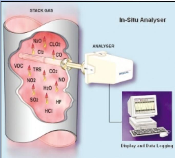
Procal Analytics Ltd have been supplying continuous monitoring systems into the Nitric Acid industry for over 20 years. The instruments are designed to withstand the harsh environment with minimum maintenance requirements. The analysers are capable of monitoring up to six gas species simultaneously, displaying, data logging and transmitting the concentrations.
