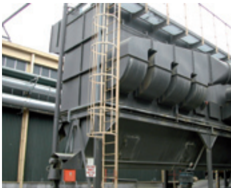
Bag House monitored by Electrodynamic® Sensors
