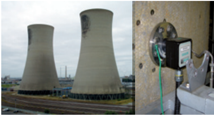
Approved (MCERTS /TUV) Dynamic Opacity Instruments monitoring the output from a Boiler Plant Electro filter on a Coal-Fired Power Plant
