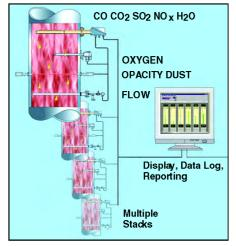
The PULSI 200 CEM system is capable of receiving data, in the form of 4-20mA signals, from other instruments. These typically measure parameters such as: Oxygen Opacity/Dust and Velocity. In addition to displaying, data logging and retransmitting this the PULSI 200 system can use this data to correct the readings to a normalised level such as 11% Oxygen. The PULSI 200 measures the water content of the stack gas and can therefore display the measured component on either a wet or dry basis.
