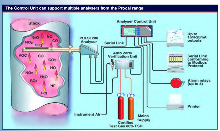
The selected infra-red wavelengths (8) used for analysis are obtained by means of interference filters and gas filled cells mounted on a rotating wheel located in the STACK MOUNTED ANALYSER.
