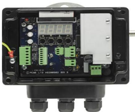
The instrument supports internal electronic self-checks as options. For added benefits, these may be upgraded from manual to automatic control.
